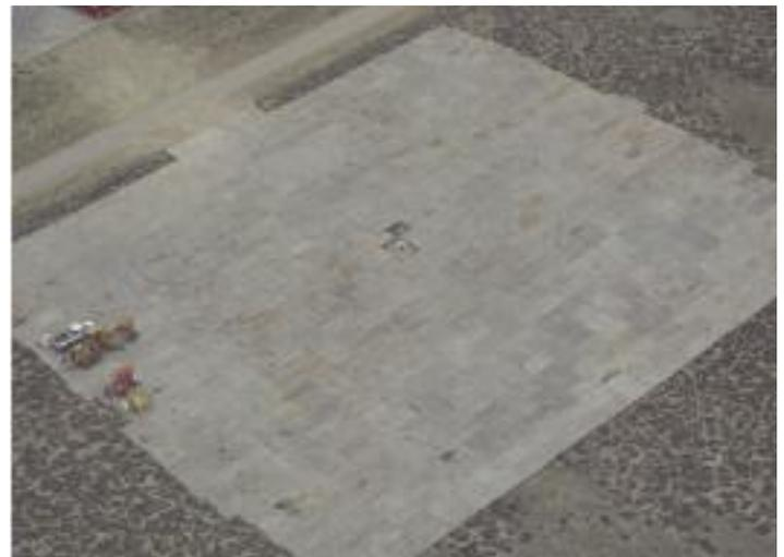
Figure 55. Mat drilling pad in the Jonah Field south of Pinedale, WY. (Photo courtesy of BLM, Pinedale Field Office).
