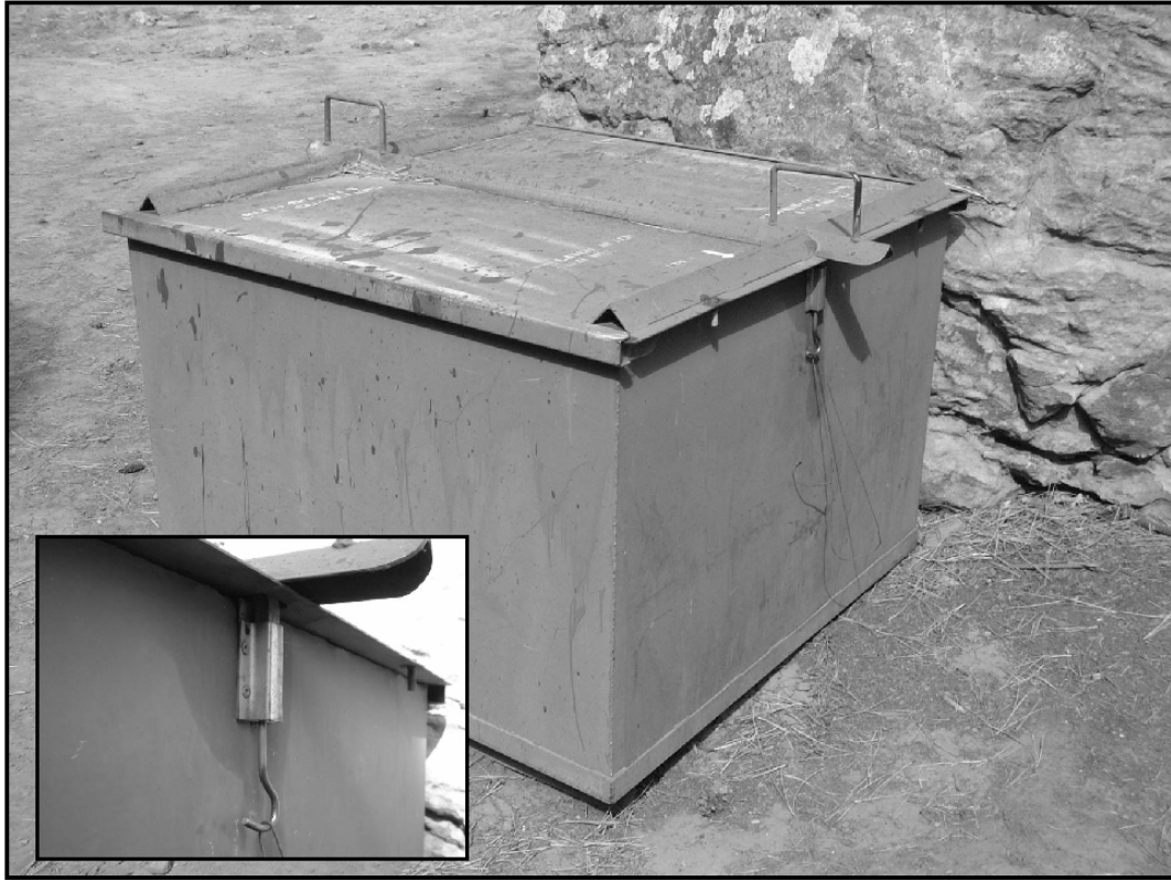
Figure 3. Bear-proof container used for storing garbage, food, or animal feed, Philmont Scout Ranch, New Mexico. The lid is secured by a spring-loaded peg that fits into a hole drilled into the edge of the lid and is released by pulling down the spring using the hook (inset).
