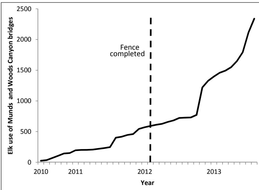
**Figure 6.** Cumulative number of elk crossing under Munds and Woods Canyon Bridges before (19 months) and after (19 months) a fencing retrofit to exclude elk from a 9.17 km section of Interstate-17 and connect existing structures from July 2010- August 2013, Arizona, USA.
