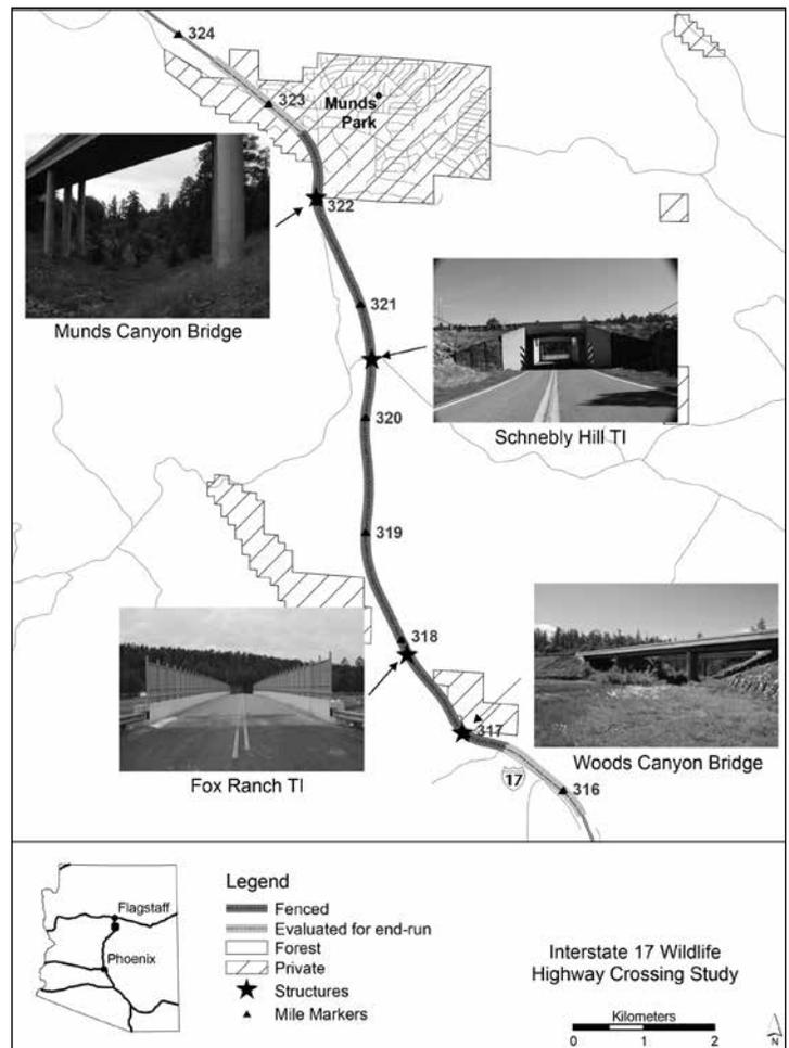
**Figure 3.** Map showing location of existing structures linked with 9.17 km of heightened right-of-way fence to reduce elk–vehicle collisions, and adjacent land ownership along Interstate-17 in northern Arizona, USA (completed February 2012). TI = traffic interchange.
