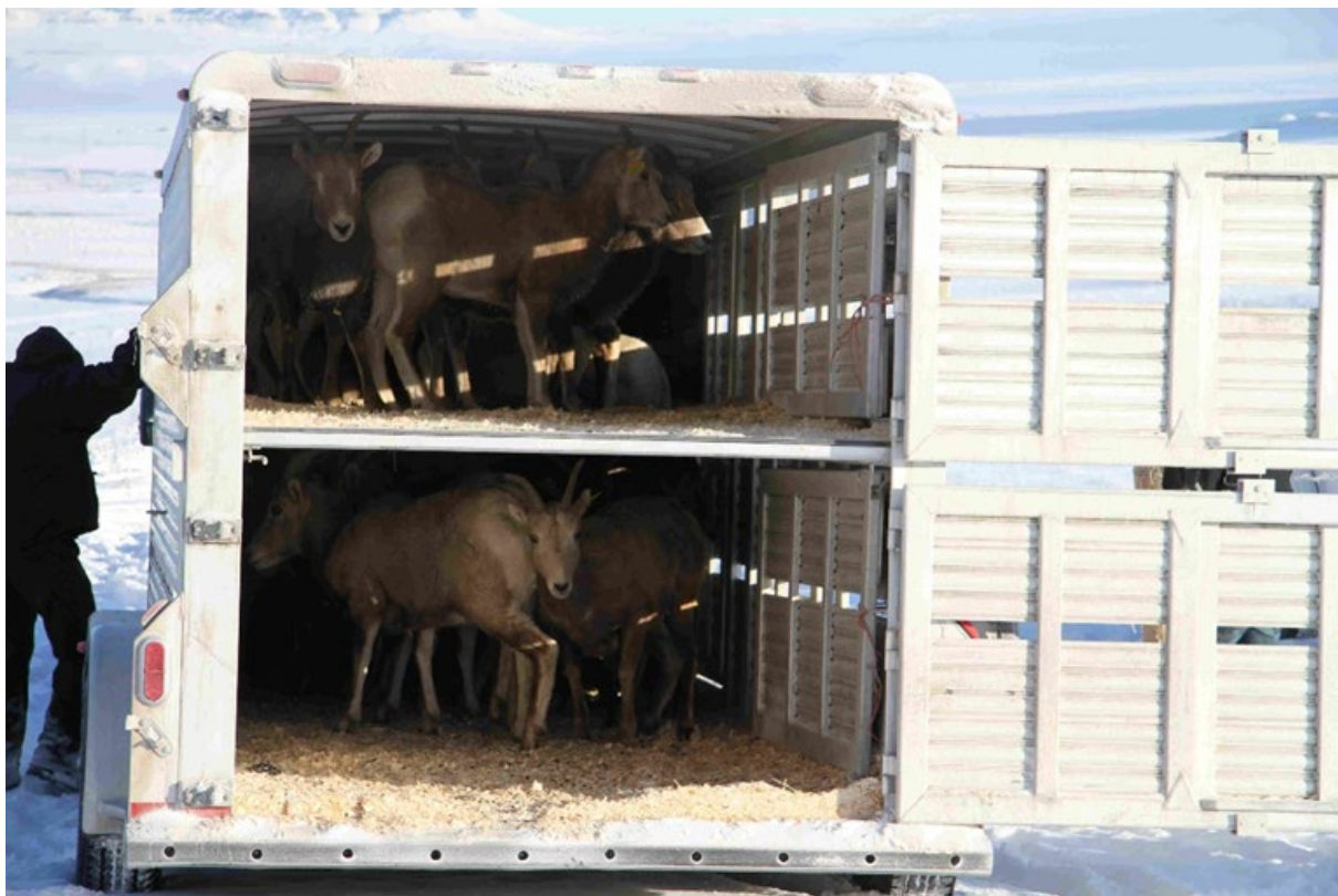
Figure 9.3. Sheep transport trailer with upper and lower decks including swinging center dividers.
