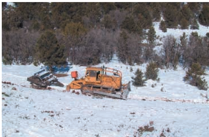
Figure 19. Roller choppers offer a more affordable method of mechanically treating large areas. (Photo by Bruce Watkins/CDOW).
