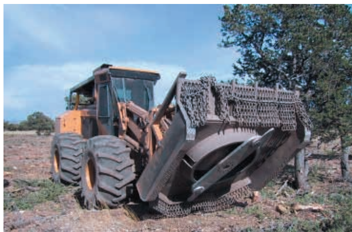
Figure 19. Roller choppers offer a more affordable method of mechanically treating large areas. (Photo by Bruce Watkins/CDOW).
