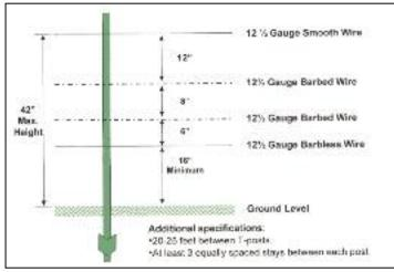
Figure 10. Specifications for a 4-strand, wildlife-friendly fence. Modification to existing fences can be accomplished by either removal of the bottom wire of an existing 4-strand fence or replacement of the bottom wire with a smooth wire that is  $\geq$ 16 inches off the ground allowing for deer fawn (and pronghorn) movement.
