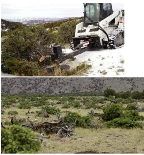
Figure 85. Hydro-axe mounted on a bobcat compact track loader (upper photo) causes very little soil disturbance and can be used on top of snow in the winter to lessen soil disturbance to cut pinyon and juniper trees flush with the ground. The lower photo is the result of the hydro-axe in felling trees on a moderately dense P-J stand. (Photos courtesy of Kreig Rasmussen/USFS – Fishlake).
