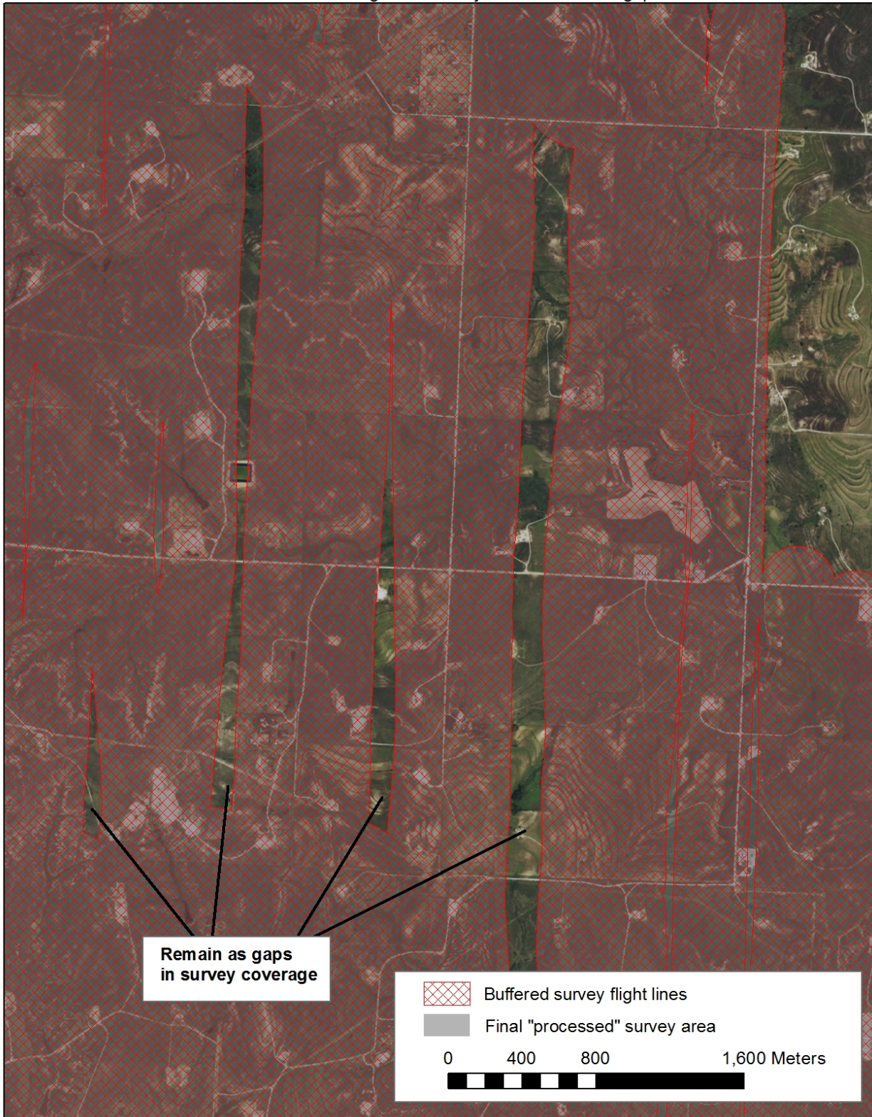
Figure 4. Buffered aerial surveys with both small sliver gaps and a large un-justified gaps. The larger gaps here will not be considered as surveyed areas.
