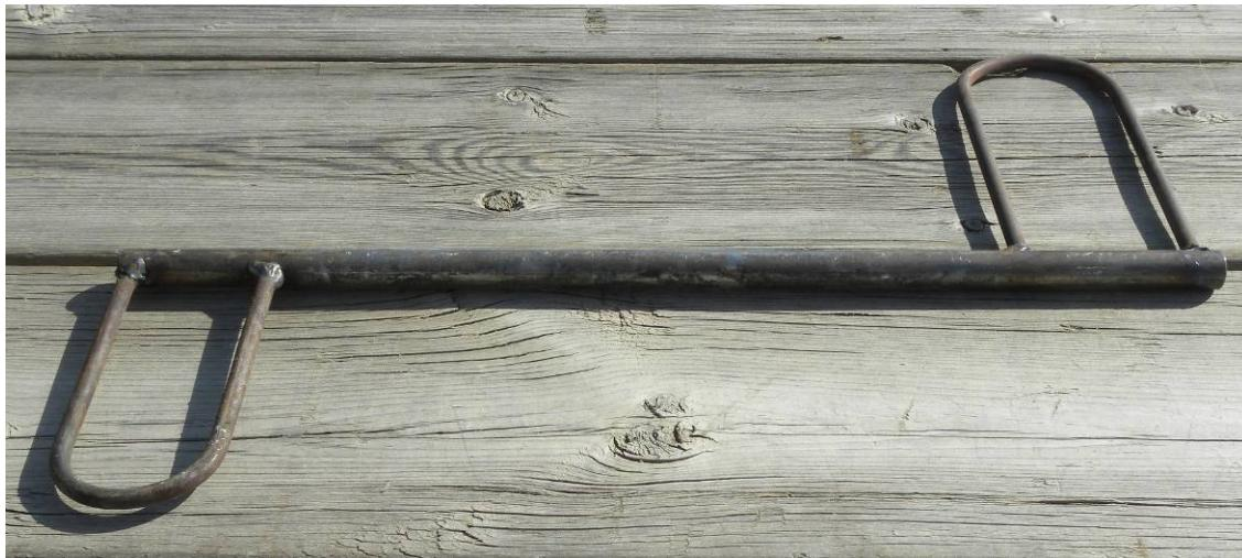
Figure 10. This simple jaw spreader allows biologists to quickly and easily pry open a deer's mouth to examine tooth eruption and wear. The smaller end (approx. 2.75 x 5.5 in [7 x 14 cm]) is used for deer and the larger end (approx. 3.5 x 7 in [9 x 18 cm]) for elk. Overall length is approximately 20 in (51 cm). Photo by T. Keegan, IDFG.
