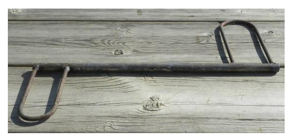
Figure 10. This simple jaw spreader allows biologists to quickly and easily pry open a deer's mouth to examine tooth eruption and wear. The smaller end (approx.  $2.75 \times 5.5$  in [7 x 14 cm]) is used for deer and the larger end (approx.  $3.5 \times 7$  in [9 x 18 cm]) for elk. Overall length is approximately 20 in (51 cm). Photo by T. Keegan, IDFG.
