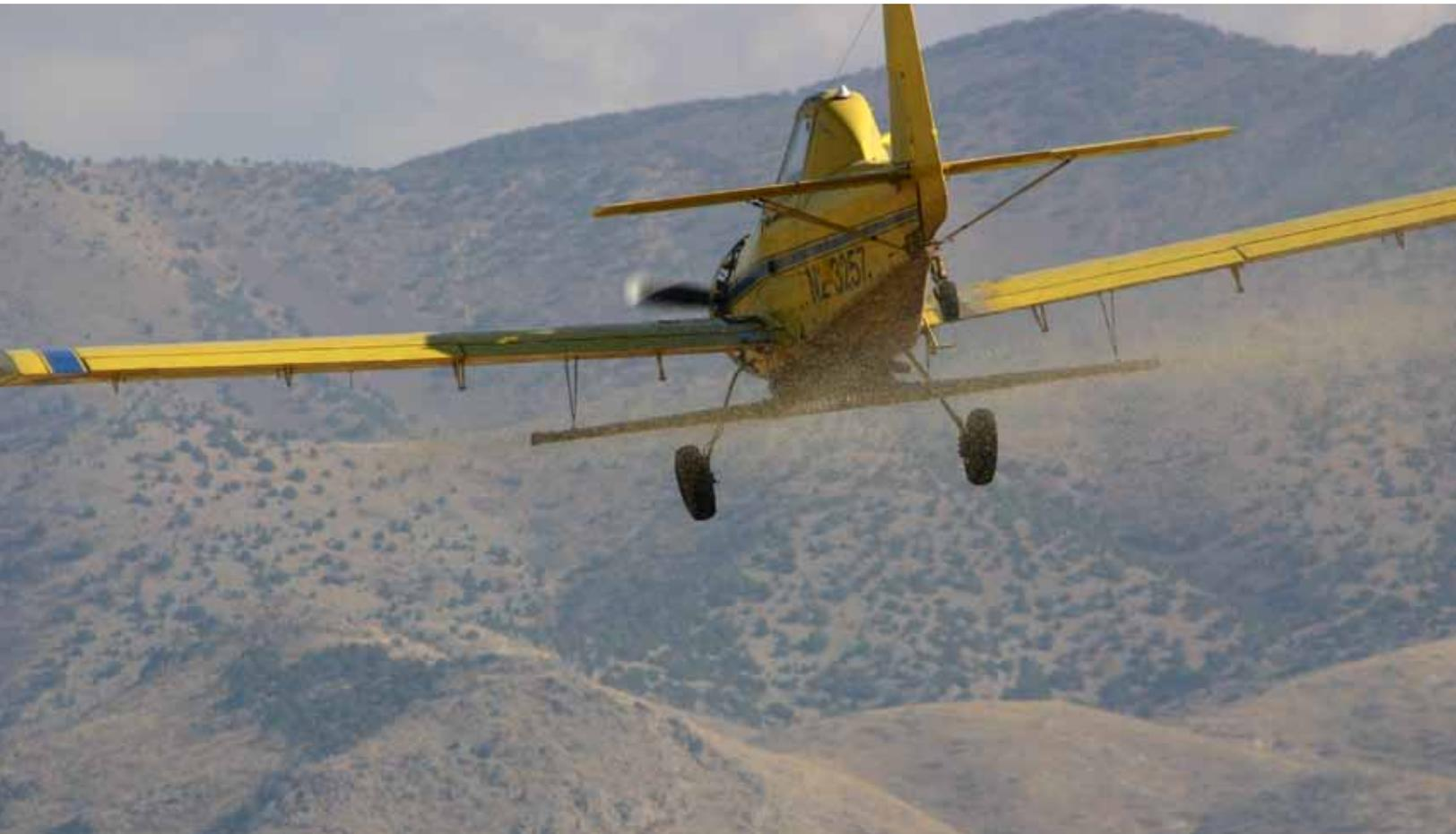
*Figure 24. Aerial seeding using fixed wing aircraft. (Photo courtesy Utah Watershed Restoration Initiative)*
