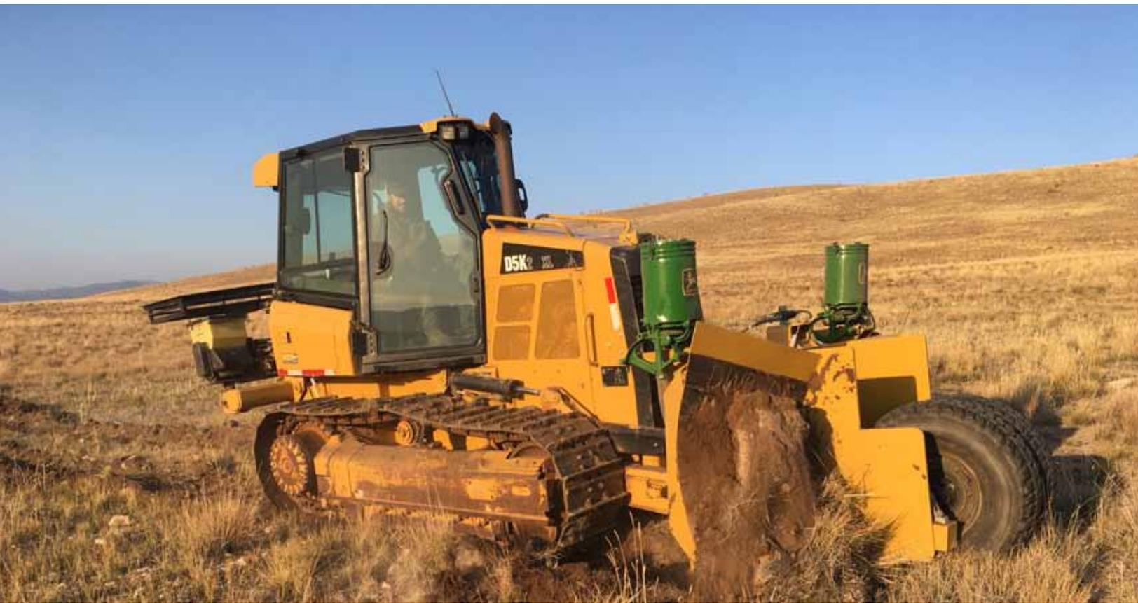
*Figure 20. Modified bulldozer for interseeding in grass dominated slopes. (Photo by Daniel D. Summers/UDWR).*
