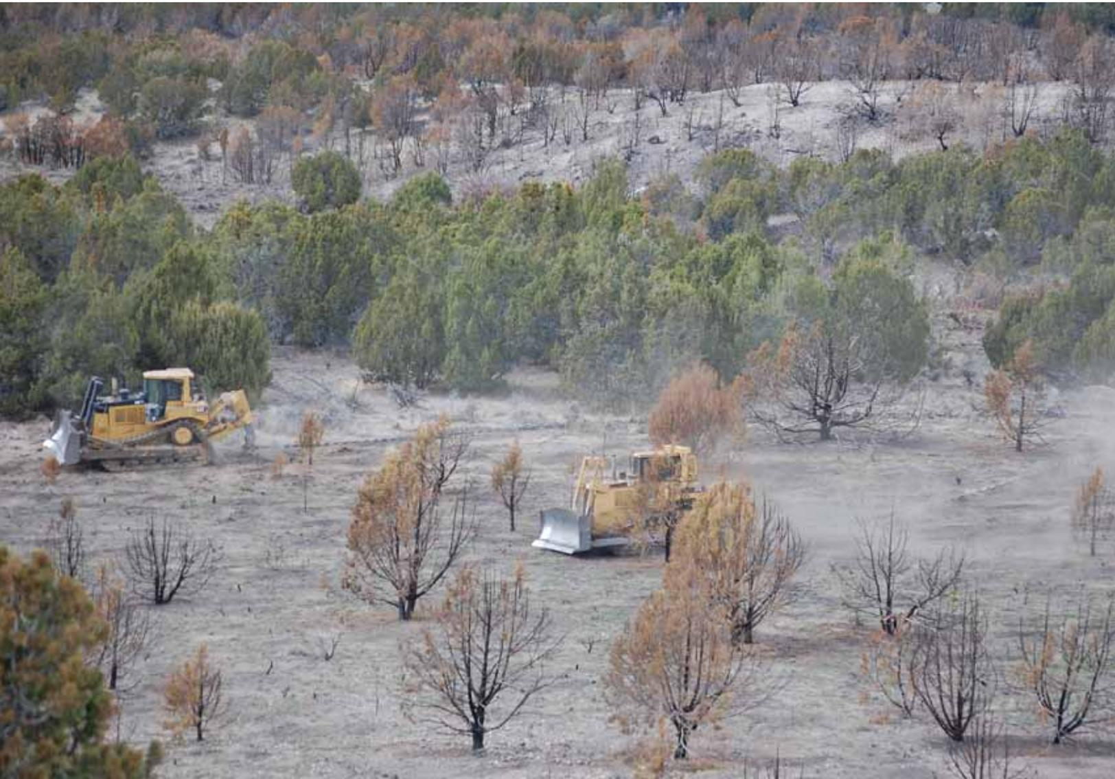
*Figure 23. Bulldozers pulling an anchor chain to cover aerially broadcast seed after a wildfire. (Photo by Daniel D. Summers/UDWR).*
