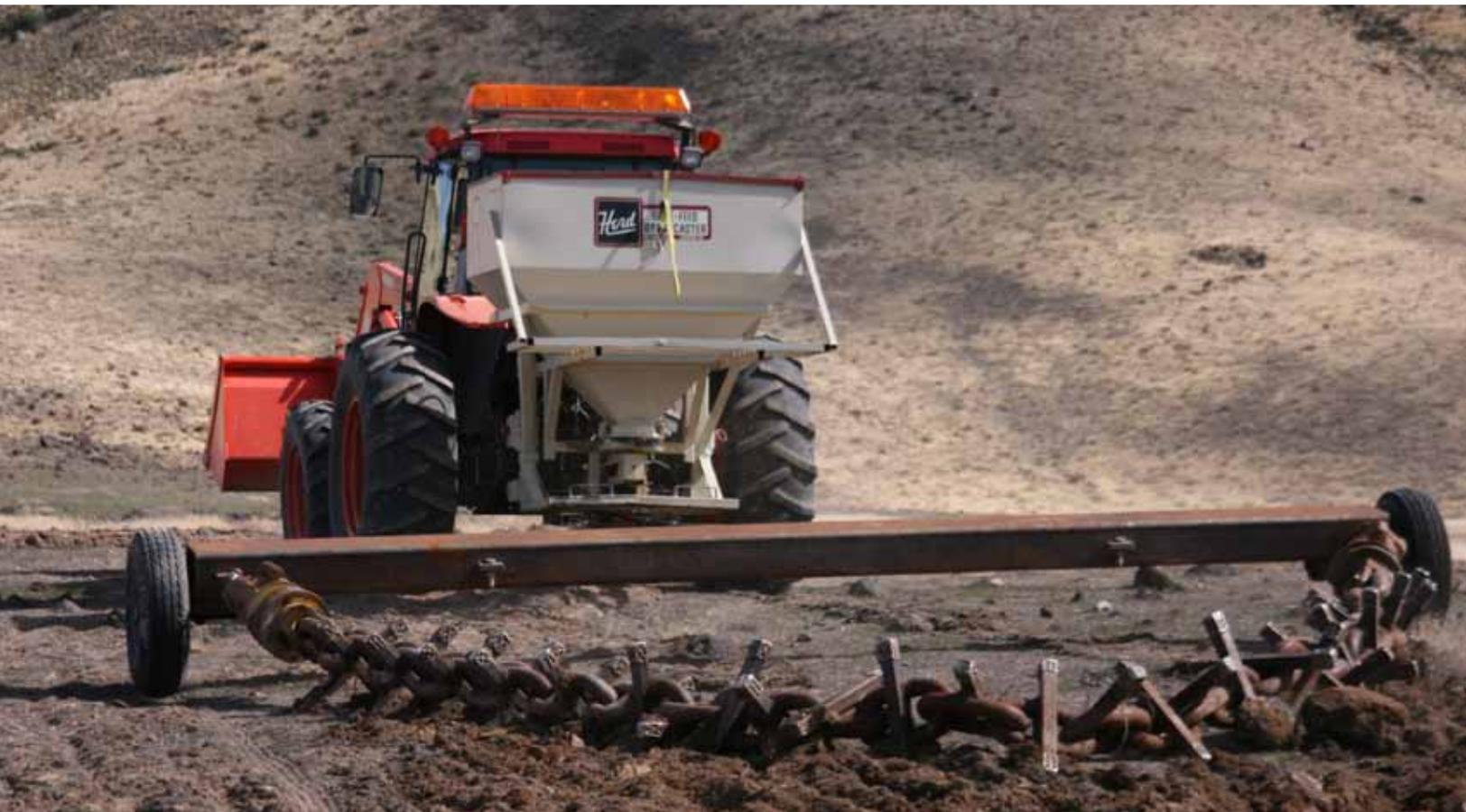
*Figure 14. Tractor mounted broadcast seeder and chain harrow to cover seed. (Photo by Daniel D. Summers/UDWR).*
