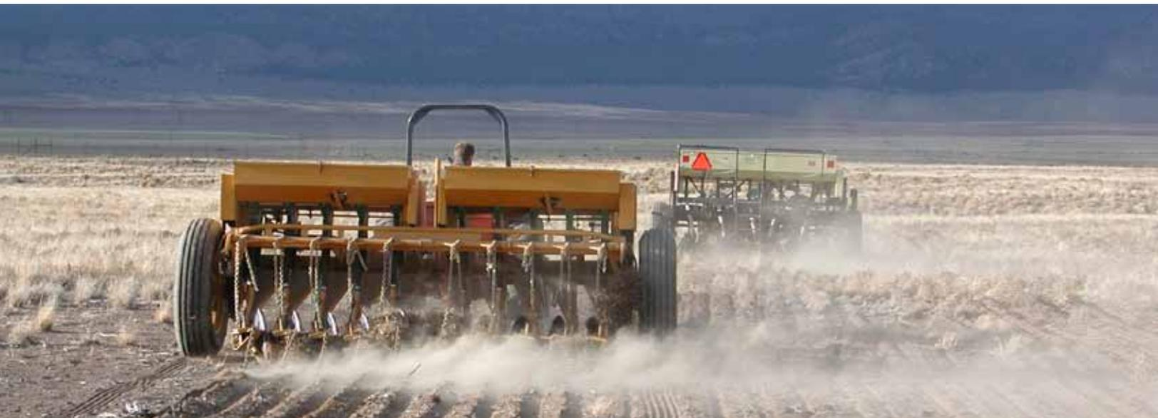
*Figure 22. Rangeland drill (left) and no-till drill (right). (Photo by Jason L. Vernon/UDWR).*
